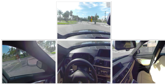
Figure 2: View from inside the simulation, each frame represents the participant’s view as they turn their head to look around, illustrating the 360-degree view inside the VR simulator.
